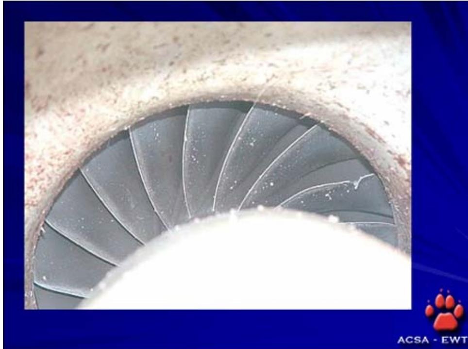
The turbobfan blades visible through the engine turbo air intake shows some damage and bird debris is visible all throughout the air intake cowling and inner surface.
