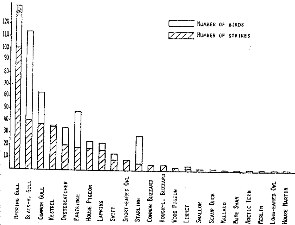
Fig. 2. The frequency of strikes per species 1974-83. Some strikes include two or more individuals and therefore in some species the number of identified birds exceed the number of strikes.
