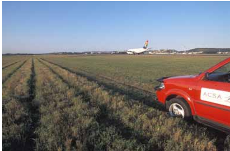
Figure 3. Bird scaring patrols are conducted from a grass track alongside the runway (50m away) outside of the runway strip / manoeuvring area.
