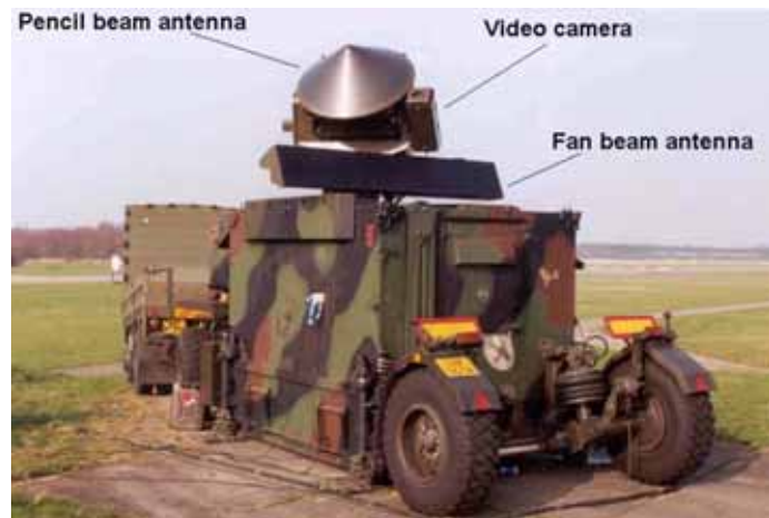
Figure 3. The mobile tracking radar with a fan beam for searching and a pencil beam for tracking birds
